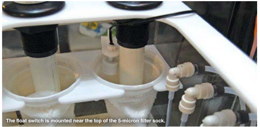
The phosphate remover is added to the system water using this mixing tee (before emptying into the filter sock).
